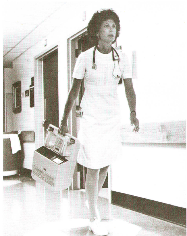
Fig. 10. The 78660A can be quickly detached from its 78668A Quick-Mount Power Base and easily carried to a cardiac emergency. All of the necessary cables, electrodes, and recording paper are contained in the instrument.
